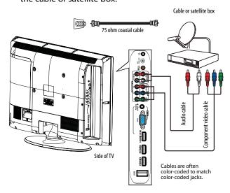
**4** Connect an audio cable (provided) to the **L** and **R** audio jacks on the side of your TV and to the audio out jack on the cable or satellite TV box.
